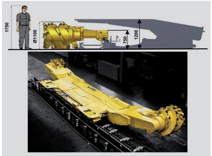
**Fig. 6:** Compact shearer loader SL 300L – face thickness 1.2 - 1.8 m
