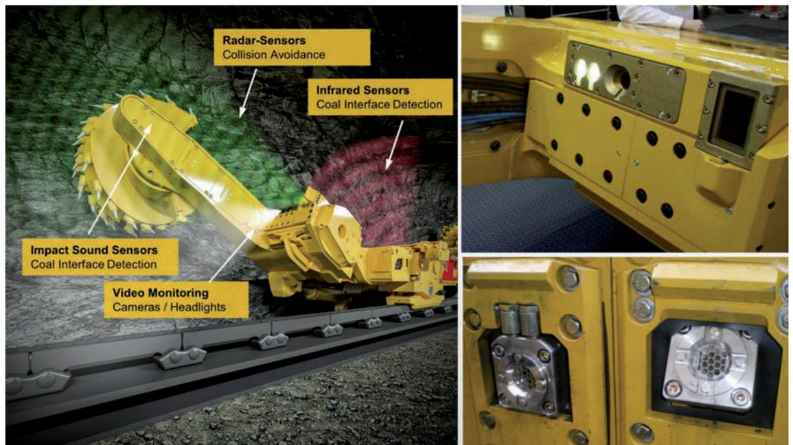
**Fig. 4:** Environment detection systems on the shearer loader
