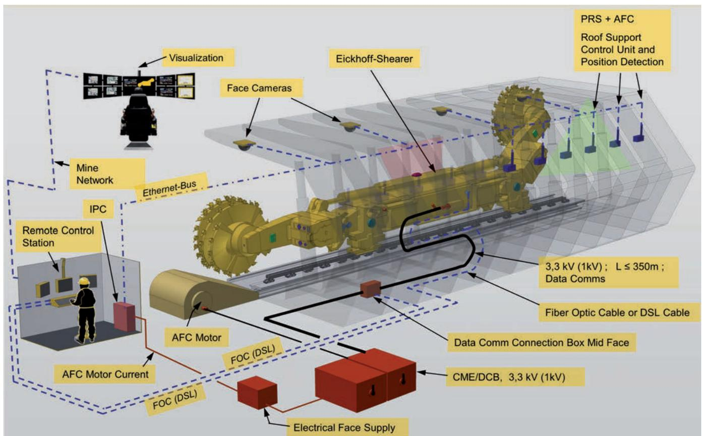
**Fig. 5:** The shearer loader as a central element in the longwall
